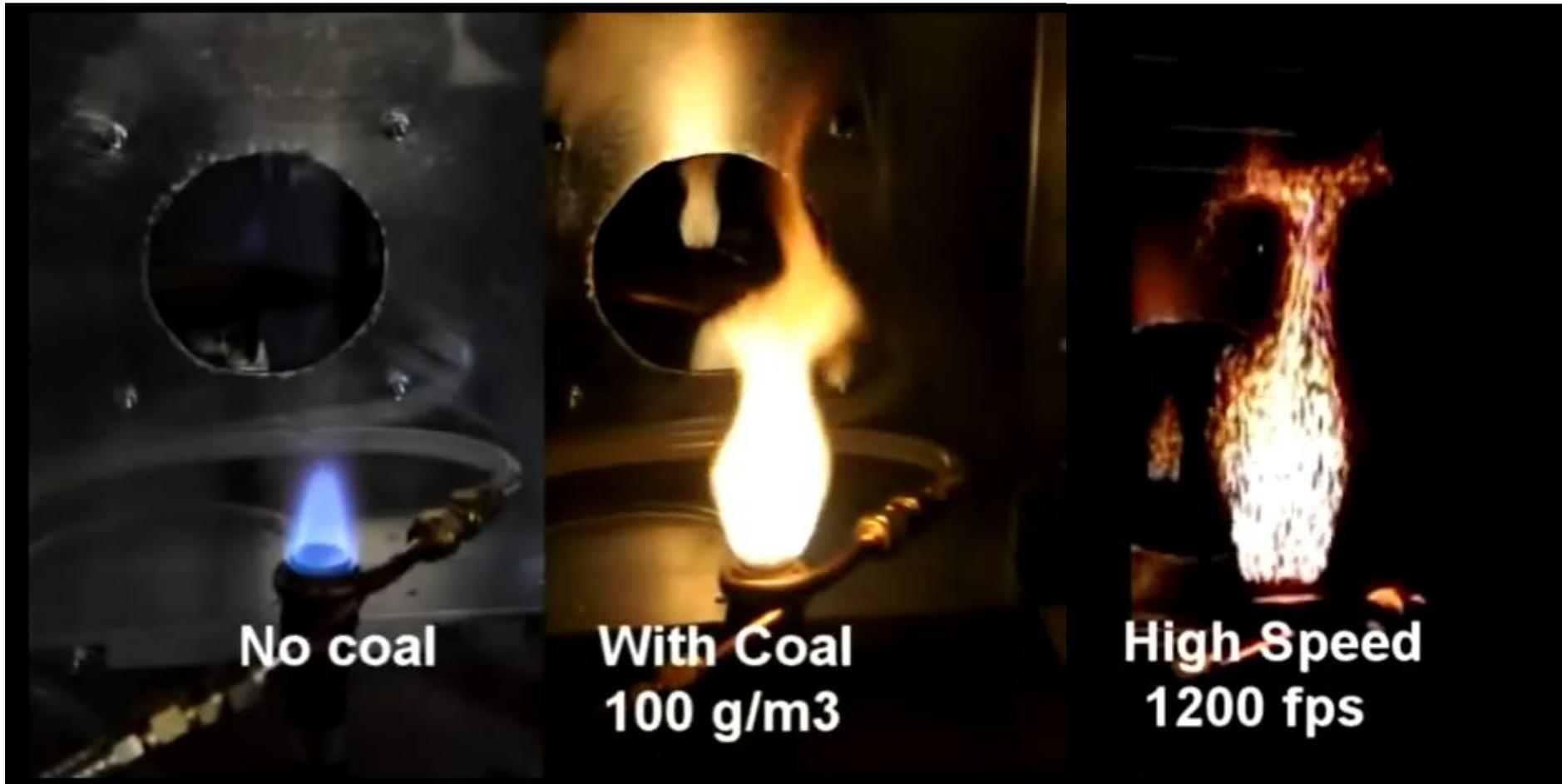
Coal particles (75-90 micron) are fed into a premixed methane air flame at a rate of  $100 \text{ g/m}^3$ .
