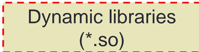
*Dynamic linking at runtime, no libraries contained in the executable and these are loaded in when the program runs*
