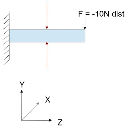
Figure 1: A cantilever beam model
