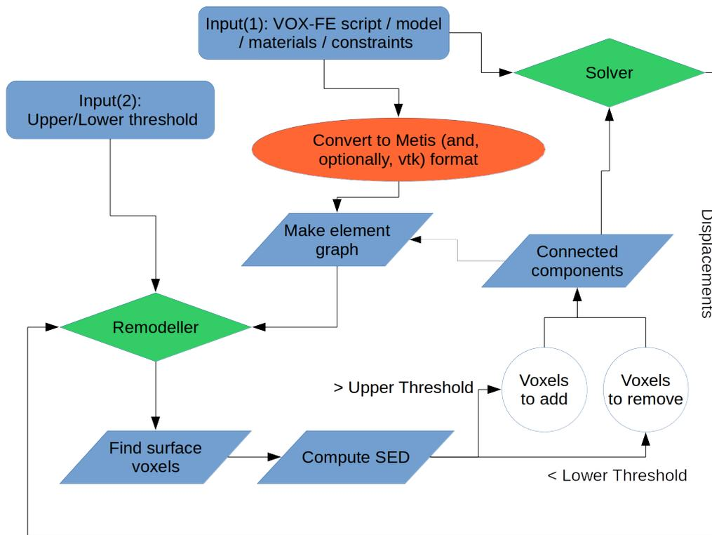
Figure 6: Workflow diagram of remodelling
