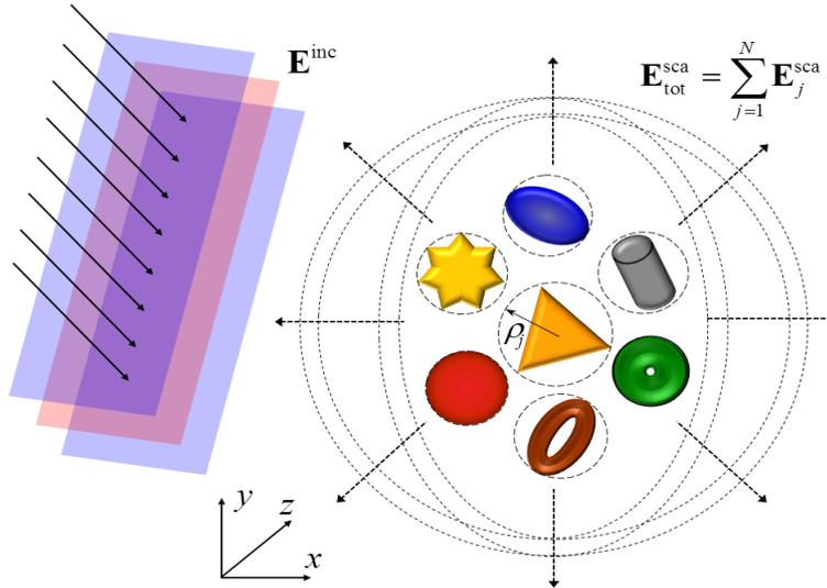
**Figure 1.** Schematic representation of the incident field/scattered field theoretical model and 3D structure of a cluster of arbitrary scatterers.
