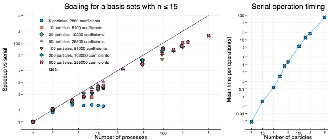
**Figure 6:** Performance of OPTIMET when the iterative solver GMRES from Trilinos in conjunction with the Decomposed Sparse Matrix-Vector Operation. The left panel shows the speedup achieved with respect to the serial code. The right panel shows the time taken by the serial code with respect to the number of particles.
